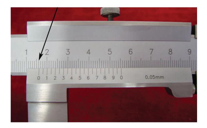
c. Look along the ten marks on the vernier scale and the millimeter marks on the adjacent fixed scale, until you find the two that most nearly line up. (0.25mm on the vernier scale)
