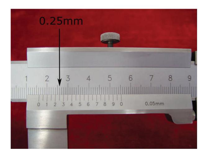
d. To get the correct reading, simply add this found digit to your previous reading. (10mm + 6mm + 0.25mm= 16.25 mm)
